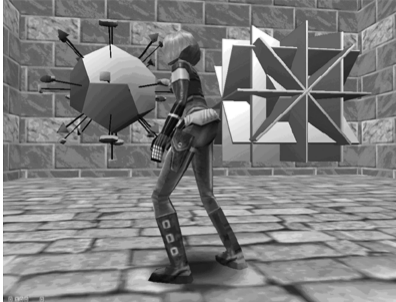
Fig.3. 3-D animated rhombic dodecahedron crystal models showing three tetrad, six diad, four triad axes and nine planes of symmetry with voice description. Note: axes of symmetry to the left and planes of symmetry to the right.
